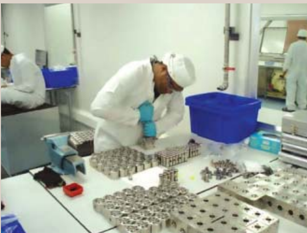
DCV valve assembly in Aker Kvaerner's Port Klang facility.
