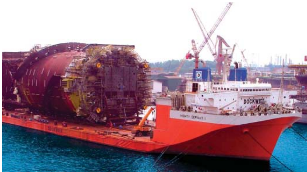
The Spar hull was loaded onto heavy transport vessel, The Mighty Servant 1, and sailed to Kikeh site on September 26, 2006
