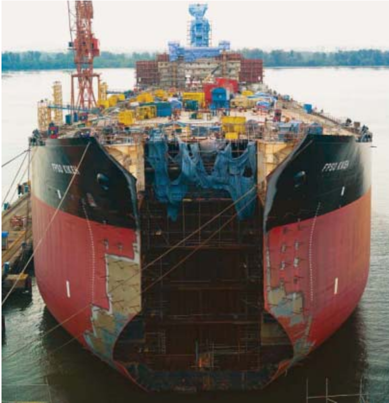
FPSO Kikeh was converted at the MMHE shipyard in southern Peninsular Malaysia
