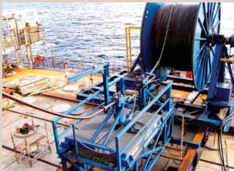
Where crane lift capacities limit the size of CT reels, BJ DuraLink connectors offer an economical way to enter deep or extended-reach wells.
