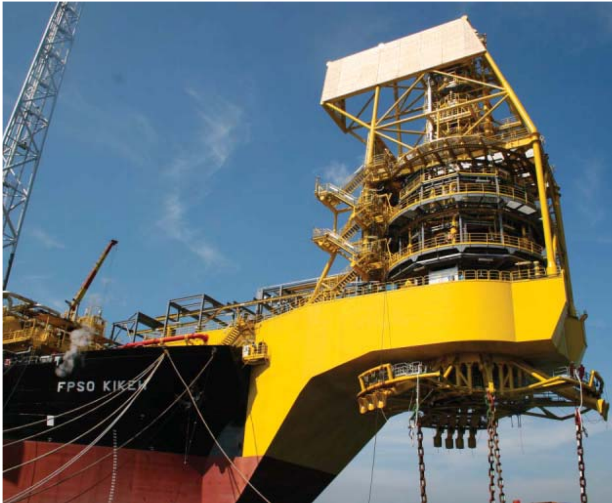
The first turret-moored FPSO used in conjunction with a Spar
