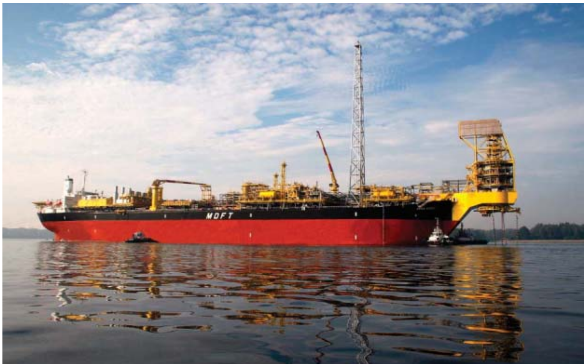
The FPSO is the central processing facility for Kikeh measuring 367m in length, breadth of 55m and weighs 273,000 tons
